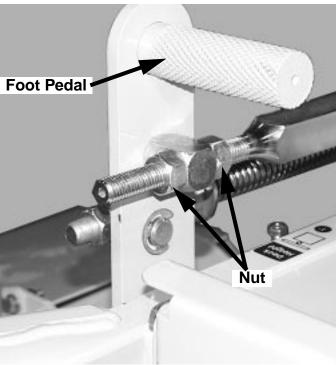
Deck Level Adjustment Foot Pedal Figure 3-19
